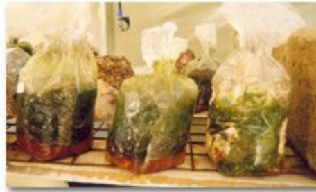
Figure 6. Bags contaminated by green and black mould
